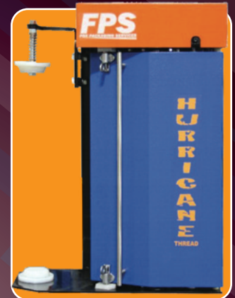
POWER DE-ENERGIZED WHEN CARRIAGE DOOR OPEN
